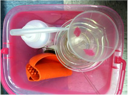
2 cans per table, in each: Scoopula Clay triangle Test tube tongs Beaker tongs Wire gauze Crucible Tongs <u>2 baskets;</u> 1 of each:
